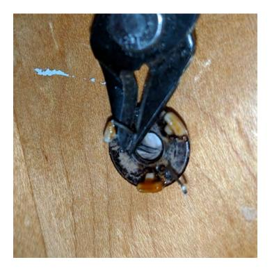
4: snip both wires as close to the ceramic base as you can and free the ceramic disk.
