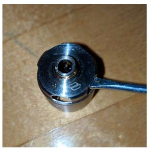
3: Gently push down on the coil and remove it from metal case.
