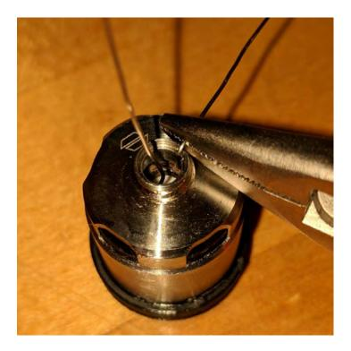
9: Pinch the wire in the slot and roll your pliers to apply pressure to the wire. You don't need a lot but enough to keep the coil in place. You want the wire to bend into the slot. Do not apply any pressure to the other wire that you bent 90°.
