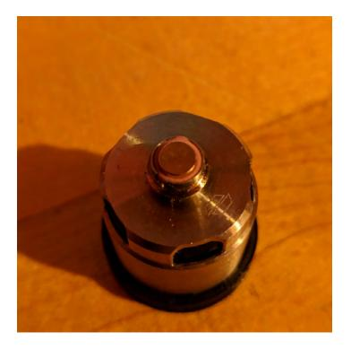
12: Put the gold pin in making sure the wire stays on the opposite side as the wire you put in the slot. The pin must be in contact with the wire.
