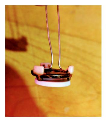
7: Put the assembled coil into the jig and bend on wire 90° towards the center then 90° straight up. The other lead is bent 10° towards the center then straight up.
