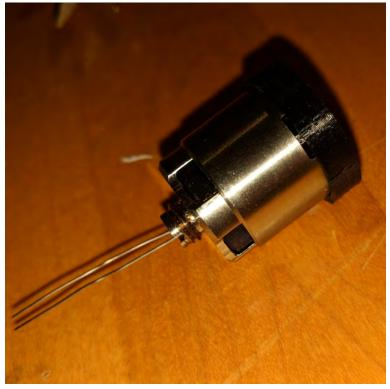
8: Gently slide the metal case over the coil/jig making sure to align the wire that was bent 10° to the slot in the threaded section. The black plastic should be touching the bottom of the metal casing like shown in the picture.
