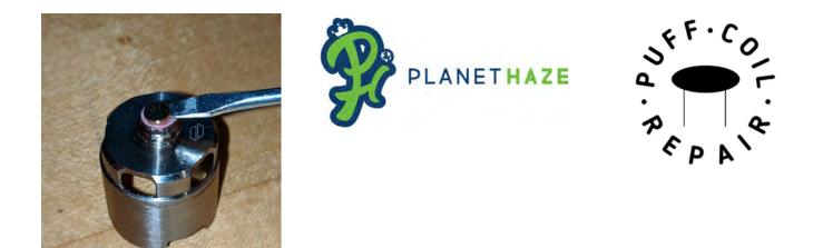
1: Pry centre pin out with small screwdriver, be careful not to damage pink grommet we'll be using this later.
