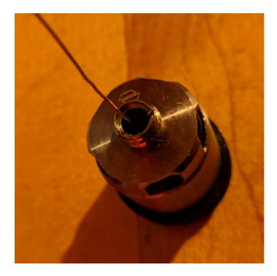
10: Cut the wire as close to the threads as you can.
