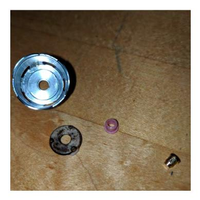
5: Clean all the parts pictured really well with isopropyl alcohol and qtips. Scrap the ceramic base clean with a razor.
