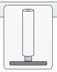
If your extract is in a vial, place the vial into the Fill Tool upside down and with the cap off (3a). If your extract is not in a vial, just load it directly into the Fill Tool (3b).
